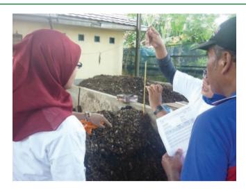
**Case Study 15.3 Figure 4** *Monitoring of the compost temperature at the Material Recovery Facility.*
